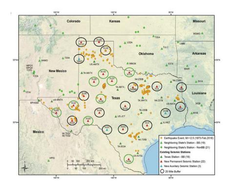
**FIGURE 3-11** In 2015, the Texas Legislature provided funding for installation of the TexNet seismic monitoring system to improve statewide seismic monitoring capability by increasing the number of seismic stations in Texas from 18 to 43. Stations with green circles are currently being installed. SOURCE: BEG, 2016.
