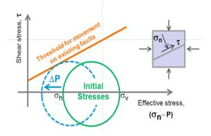
**FIGURE 3-9** Illustration of subsurface pressure and stress conditions that are associated with fault stability and fault slip. SOURCE: Ground Water Protection Council and Interstate Oil and Gas Compact Commission. 2015.
