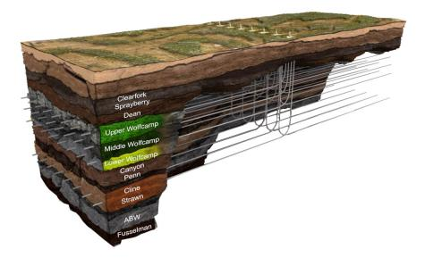
FIGURE 2-6 Diagram showing pad well drilling concept. Each well will have roughly uniformly spaced hydraulic fractures created perpendicular to the horizontal well segment.
