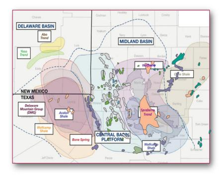
**FIGURE 2-2** Conventional reservoirs (small outlined shapes) overlying known shale resource plays (large pastel-shaded regions) in the Permian Basin near Midland, Texas. Wells located in any of the shaded plays may profitably produce oil for a sufficiently high oil price. SOURCE: EPT.
