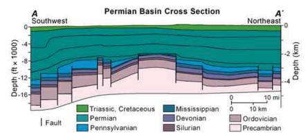
**FIGURE 3-3** Cross section of the Permian Basin of Texas. Section A-A' spans the deep Delaware Basin, high Central Basin Platform, and moderately-deep Midland Basin provinces of the Permian Basin. The Permian age sediments vary in thickness from 11,500 feet in the Delaware Basin to 5,000 feet on the Central Basin Platform. Oil and gas have been produced from each of the formations located between the Triassic/Cretaceous surface down to the Precambrian basement. SOURCE: BEG, 1990.
