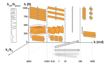
**FIGURE 2-3** Modern well designs. Grey cylinders are wells, and orange planes are hydraulic fractures. The red outline indicates well designs of interest for this report. The symbols are h for formation thickness, k for permeability (md is millidarcy); subscripts are v for vertical, h for horizontal, net for producible pay out of a total gross pay thickness. SOURCE: EPT. 2015.
