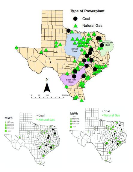
**FIGURE 5-4** Locations of coal-fired and natural gas-fired power generation relative to oil and gas production regions in Texas (top panel). Distribution of electricity generation at high natural gas prices (sizes of dots representing power plants is proportional to extent of generation; bottom left panel). Distribution of electricity generation at low natural gas prices (sizes of dots proportional to extent of generation; bottom right panel).
