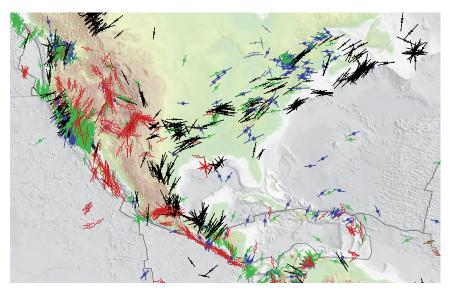
**FIGURE 3-5** World Stress Map data, illustrating the direction of the greatest horizontal stress field across the United States. The red stress orientations correspond to normal faulting regimes, green to strike-slip faulting, and blue to thrust faulting. The sparseness of data across the mid-continent of the United States creates uncertainty in understanding stress fields at smaller scales. SOURCE: Heidbach et al., 2009.
