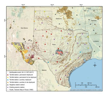
**FIGURE 3-1** Map of Texas and surrounding states showing earthquakes from the USGS earthquake database, existing and proposed TexNet seismic stations, and structure of key stratigraphic units portraying the complex tectonic architecture and fault systems in Texas.
