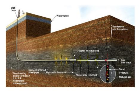
**FIGURE 2-4** Diagram showing hydraulic fractures in a horizontal well drilled into a shale formation. SOURCE: Ryerson, 2014.
